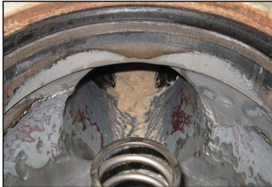
Worn coating exposes metal in <3000 hours
